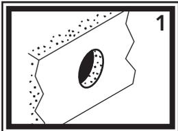
1) Hold elbow on the wall where desired. Make sure to leave enough room for the hose to hang freely and extend into the shower. Drill 1" hole in the bulkhead in the desired location.
