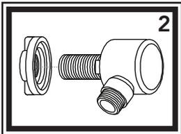
2) Make sure male nipple is tight into the elbow with Teflon (Plumber's) tape. Slip nipple through the hole in the bulkhead. Make sure gasket properly lines up with the back of the elbow. From the back side of the bulkhead, thread the lock nut onto the brass nipple and tighten.
