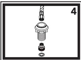
4) Slide hose/sprayer assembly back through the hose nest shaft from above the deck and replace the 1/2" adapter.
