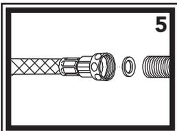
5) Connect to desired 1/2" NPT-Male water source or valve. Make sure the rubber washer is in place in the larger female side of the adapter.
