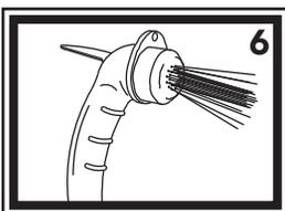
6) This sprayer has two functions: intermittent and continuous. For intermittent spray, simply press down on the trigger. For continuous spray, lift up on the trigger until it locks. To release, simply press the trigger back down. If you wish to remove the hook from the sprayer, unscrew the face. Slide the hook off the sprayer and remove the large, black, flat washer from inside the face. Replace the face.
