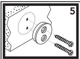
5) Mount the bracket as shown. For mounting into fiberglass or other solid surface, drill a 1/8" starter hole and attach the bracket to the wall.
