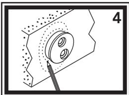
4) Hold the bottom post on the wall where desired. With a pencil, lightly trace a circle completely around the base of the post. Remove the post. Hold a mounting bracket directly in the center of the outline. Trace a circle around the mounting bracket and the two mounting screw holes.
