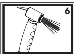
6) This sprayer has two functions: intermittent and continuous. For intermittent spray, simply press down on the trigger. For continuous spray, lift up on the trigger until it locks. To release, simply press the trigger back down.
