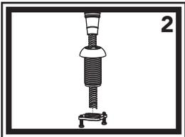
2) Remove holder assembly from hose/sprayer assembly. Unscrew the lock nut with the screws from the mounting shaft.
