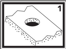
1) Check desired position to make sure there is enough room for the hose to gather under the deck without getting caught on anything. Drill 1 3/8" diameter hole (standard size) in the deck in the desired location.
