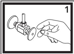
1) Turn off the water supply to your existing faucet (this procedure will vary depending on the specific plumbing system installed on your boat). Cover the sink drain to prevent any small parts or debris from falling in. Remove your existing faucet, taking care not to damage your existing water lines. Clean sink area in preparation for new faucet.
