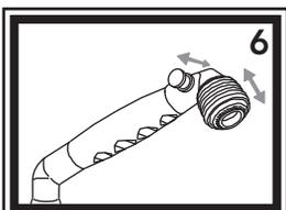
6) To switch from normal aerate to spray, simply pull down on the chrome ring around the aerator. Push it back up to switch back to aerate from spray. To set the faucet to "stand-by" push the stand-by button on the head of the sprayer. Push the button on the opposite side of the sprayer to allow water to flow. NOTE: "STAND-BY" WILL ALLOW A SMALL AMOUNT OF WATER TO CONTINUE TO TRICKLE OUT OF THE SPRAYER.
