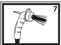
6) Set sprayer in bulkhead bracket. Push down on the sprayer slightly to insure that it is resting securely in the bracket.
