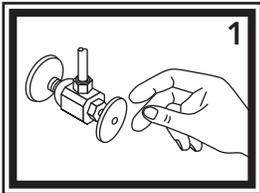
1) Turn off the water supply to your existing faucet (this procedure will vary depending on the specific plumbing system installed on your boat). Cover the drain to prevent any small parts or debris from falling in. Remove your existing faucet, taking care not to damage your existing water lines. Clean area in preparation for new faucet.
