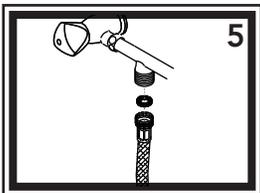
5) Attach hose to connector bar. Make sure black rubber washer is inside the fitting on the hose before attaching.
