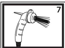
7) This sprayer has two functions: intermittent and continuous. For intermittent spray, simply press down on the trigger. For continuous spray, lift up on the trigger until it locks. To release, simply press the trigger back down. If you wish to remove the hook from the sprayer, unscrew the face. Slide the hook ring off the sprayer and remove the large, black, flat washer from inside the face. Replace the face.
