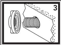
3) Slide valves into holes in the bulkhead. From the back side of the wall attach the lock nuts and tighten. Then attach water source to the 1/2" Male inlets.
