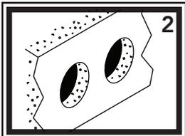
2) Hold valves and bulkhead bracket on the wall where desired. Make sure to leave enough room for your hose to hang freely and extend into the shower. Mark locations on the wall with a pencil. Drill 1" holes in the bulkhead in the desired location for the valves and 1/8" starter holes for the bulkhead bracket screws.
