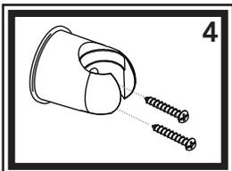
4) Mount bulkhead bracket with the two stainless steel screws provided. The top of the bracket is the side with the larger diameter opening.
