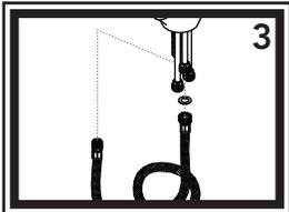
3) Connect sprayer hose to center connector hose. Wrap the brass fitting on the connector hose with Teflon (Plumber's) tape. From under the sink, insert the male end of the hose up through the mounting tube and out the top of the faucet.
