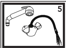
5) Before attaching the sprayer, pull the hose partially out and aim it down into the sink. Turn the water supply back on and allow both hot and cold water to run for at least one full minute without the sprayer. While water is running, check all connections for leaks. Attach sprayer to the hose. Connections may need re-tightening.
