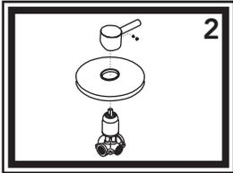
2) Remove handle and wall plate from valve assembly. Remove the blue/red cap and loosen the set screw behind it. Slide handle off the cartridge. Slide wall plate off the trim sleeve. Be careful not to damage the wall plate gasket.
