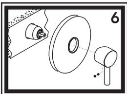
6) Replace handle and wall plate onto valve assembly. Slide wall plate back onto the trim sleeve. Be careful not to damage the wall plate gasket. Tighten the handle screw and replace the blue/red cap. It may be necessary to secure the valve inside the wall to prevent movement. This procedure will vary depending on the specific design of your boat. Suggestions: Use the screw-holes molded into the valve. Use strapping material. Wedge item in place.
