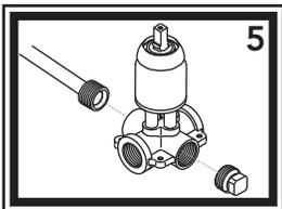
5) Connect 1/2" NPS-Male water line from the shower head or bulkhead elbow (not included) to the shower head (top) port. Wrap the fitting on the water line with Teflon (Plumber's) tape. Thread tub port plug into the tub port (bottom) (if you are not using a tub spout with this installation). Wrap the plug with Teflon (Plumber's) tape.
