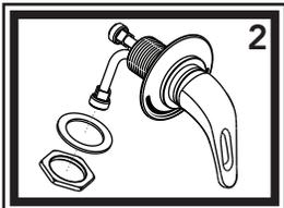
2) Unscrew the lock nut and metal washer off the back of the valve body and slide off over the copper pipes. You may need to very gently bend the copper pipes closer together to allow the lock nut and metal washer to slide over the fittings.
