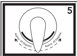
5) Ensure that when the handle is in the off position (straight down) it lines up with the marking on the wall plate. If adjustment is needed, slightly loosen the lock nut, adjust the wall plate and re-tighten.
