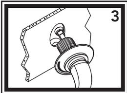
3) From the front side of the bulkhead, slide the valve assembly with the wall plate, packing rings and handle still attached, through the hole in the bulkhead.
