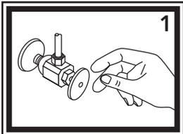
1) Turn off the water supply to your existing faucet (this procedure will vary depending on the specific plumbing system installed on your boat).
