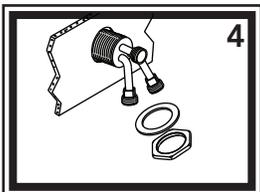
4) From the back side of the bulkhead, secure shower mixer by sliding the metal washer and lock nut back on over the copper pipes. Tightening against the back side of the bulkhead.
