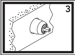
3) From the back side of the bulkhead, slide the valve assembly through the hole in the bulkhead. Note that the brass valve is stamped with "UP". Make sure that the "UP" is on the top side when positioned.
