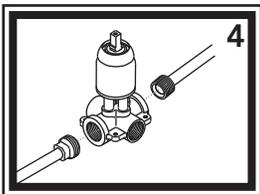
4) Connect hot/cold water supply lines (not provided) to the inlet tubes. The inlet tubes are the 1/2" NPS-Female tubes on the left and right sides of the valve. Wrap the fittings with Teflon (Plumber's) tape. This procedure will vary depending on the specific plumbing system installed on your boat.
