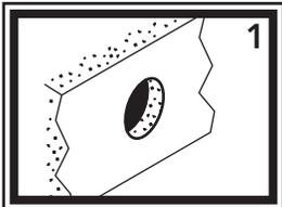
1) Check desired position to make sure there is enough room inside the wall for the valve body, connector hoses and connections. Drill a 1 5/8" to 1 3/4" diameter hole in the desired location.
