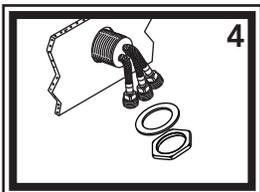
4) From the back side of the bulkhead, slide the metal washer, then the lock nut up over the connector hoses and onto the valve body. Loosely tighten the lock nut.
