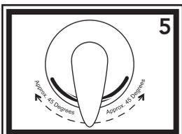
5) From the front side of the wall, ensure that when the handle is in the off position (straight down) it is centered between the hot and cold side-to-side rotation. Rotate the wall plate so that the red and blue stripe properly align with the handle. Once centered, firmly tighten the lock nut against the back side of the wall to secure.
