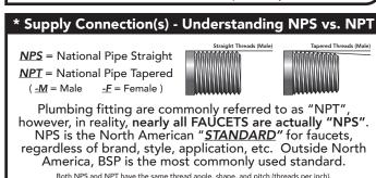
Both NPS and NPT have the same thread angle, shape, and pitch (threads per inch). However, NPS threads are straight (parallel) and NPT threads are tapered (reduced)
