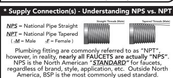
Both NPS and NPT have the same thread angle, shape, and pitch (threads per inch). However, NPS threads are straight (parallel) and NPT threads are tapered (reduced)
