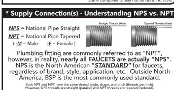
Straight Pipe thread is commonly found on faucets, showerheads, hose connections and fittings. Tapered Pipe thread is commonly found on pipe ends, nipples and fittings (i.e. couplings, elbows, tees, etc.). Straight Pipe threads need a gasket or or-ing to create a seal. Both styles require sealant or plumber's tape for optimal seal. While NPS and NPT threads will engage, they do not seal properly with each other.
