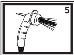
4) Connect to desired 1/2" NPT-Male water source or valve. Make sure rubber washer is in place in the female hose fitting.
