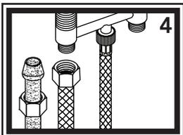
4) Connect hot and cold water supplies to the 1/2" NPT-Male inlets on the bottom of the valve. It may be necessary to use 90 degree elbow fittings, not provided. Check to ensure that the hot supply is connected to the handle with the red cap and the cold supply is connected to the handle with the blue cap.
