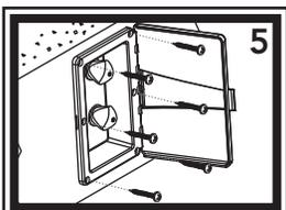
5) Carefully place the transom box and lid with all the connections securely made, back into the hole. Secure transom box and lid using the provided six (6) screws.
