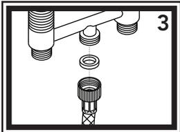
3) Connect the 72" hose to the center port on the valve connector bar. Make sure rubber washer is in place in the female hose fitting.
