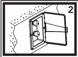
2) Set the transom box and lid into the hole to ensure proper fit and remove.
