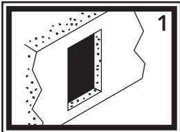
1) Check desired position to make sure there is enough room for the hose to gather under the deck or inside the wall without getting caught on anything. Cut a 4 7/8" by 7 7/8" rectangle in the desired location. Take extra care to ensure straight, clean, accurate cutting.
