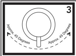
**Deck Mount**— Place into the hole with the hinge pointing in the desired direction for the lid to easily lay open when in use. Secure recessed cup and lid using the provided four (4) screws.
