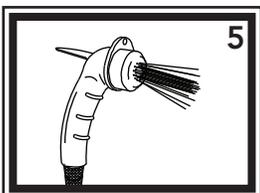
5) This sprayer has two functions: intermittent and continuous. For intermittent spray, simply press down on the trigger. For continuous spray, lift up on the trigger until it locks. To release, simply press the trigger back down. If you wish to remove the hook from the sprayer, unscrew the face. Slide the hook ring off the sprayer and remove the large, black, flat washer from inside the face. Replace the face.
