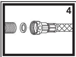
4) Connect the desired device to the 1/2" NPS-Male side port on the valve.
