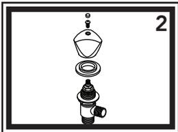
2) Remove the blue cap, handle screw, handle and escutcheon from the assembly. From the bottom / back side, insert the assembly through the hole.
