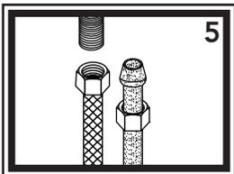
5) Connect cold water supply to the 1/2" NPS-Male inlet on the bottom of the valve. It may be necessary to use 90° elbow fittings, not provided.
