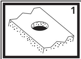
1) Check desired position to make sure there is enough room for a hose to connect to the side port of the valve, under the deck or inside the wall without getting caught on anything. Drill 1" hole in the deck / wall in the desired location.
