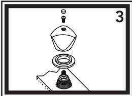
3) Screw the escutcheon back onto the valve body securely. Replace handle, handle screw and blue cap.
