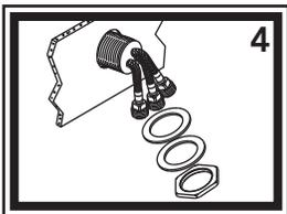
4) From the back side of the wall, slide the rubber washer, the metal washer, then the lock nut up over the connector hoses and onto the valve body. Loosely tighten the lock nut.
