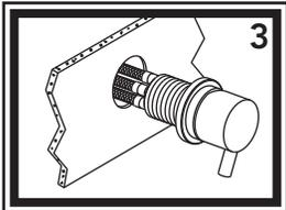
3) Slide the valve body with the three hoses attached into the hole in the wall.
