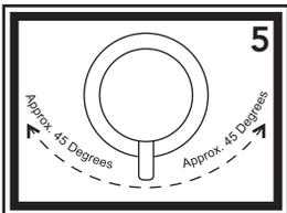
5) From the front side of the wall, ensure that when the handle is in the off position (straight down) it is centered between the hot and cold side-to-side rotation. Once centered, firmly tighten the lock nut against the back side of the wall to secure.
