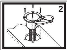
2) Place the recessed cup and lid with shut-off valve/mixer into the hole.
