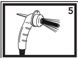
5) After installation is complete, turn the water supply back on and allow both hot and cold water to run for at least one full minute. While water is running, check all connections for leaks. Connections may need re-tightening.
