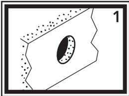
1) Check desired position to make sure there is enough room for the connector and supply hose to gather under the deck or inside the wall without getting kinked. Drill 2 7/8" to 3" hole in the desired location.
