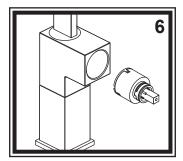
Slide the new (rotate only) cartridge into the faucet's valve body. Note that there are two alignment pins molded into the bottom of the cartridge. Make sure these pins align properly and go into their receptacles in the valve body. Proper alignment will ensure the cartridge housing is installed at the correct rotation.
