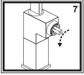
Replace the lock nut and trim cap following the reverse instructions from above. Be careful not to over-tighten the lock nut or trim cap when installing. ROTATE THE CARTRIDGE STEM TO THE "OFF" POSITION.
