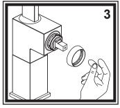
Unscrew the trim cap from the lock nut holding the cartridge in place. Be careful not to scratch the finish.
