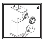
Using the adjustable wrench or pliers, unscrew the lock nut. Position the tool on the flat sections on opposite sides of the lock nut's outer threaded area. DO NOT position the tool on the threaded portion of the lock nut, as it may crush or damage the threads around the outside.
