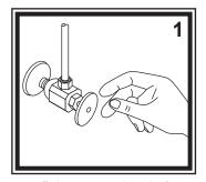
Turn off the water supply to the faucet (this procedure will vary depending on the plumbing system installed on your boat). Tilt the handle to the open position, which would normally allow for warm water, allowing any water inside the unit to drain out. Cover the sink drain to prevent small parts or debris from falling in.
