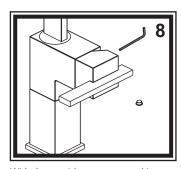
With the cartridge stem rotated into the "OFF" position, slide the handle onto the cartridge stem. The handle "blade" will be parallel to the counter top, pointing towards the front of the sink (see illustration). Using the hex wrench, tighten the set screw inside the handle. Replace the black rubber insert covering the set screw on the, now, back of the handle. Turn the water supply back on.
