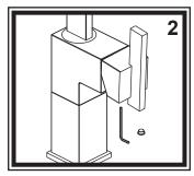
With your fingernail, pry out the black rubber insert covering the set screw on the bottom of the handle. Using the hex wrench (included), loosen the set screw inside the bottom of the handle (two or three revolutions should be enough to allow the handle to pull off the stem). It might help to rotate the handle to the back (hot) position, to give easier access to the plug and set screw. Slide the handle off the stem.
