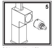
Pull the existing (tilt- on/off & rotate-hot/cold) cartridge out of the faucet.
