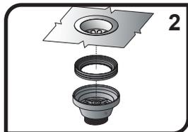
2) From under the sink, line up the Body with the Rubber Gasket with the Flange and Screw.
