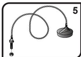
5) **OPTIONAL**- Drill a 3/16" hole in the counter-top or other surface and secure the Stopper Screw using the Stopper Nut, where desired. If you choose not to secure the Stopper Screw, you may remove the Stopper Chain from the Stopper. Spread the ends of the Stopper Triangle Connector and remove it from the Stopper.
