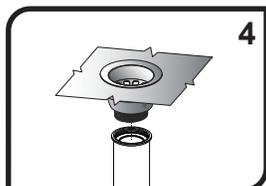
4) Screw 1 1/4" drain pipe or adapter (not included) onto the Body. Use Teflon tape (not included) on the threads to prevent leaks.
