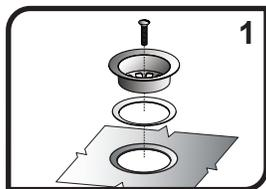
1) Set the Flange with the Foam Gasket and Screw in the drain hole in the sink. NOTE: The Foam Gasket is supplied for your convenience, however, we recommend using plumber's putty (not included) instead of the Foam Gasket. Do not use both the Foam Gasket and plumber's putty.
