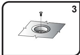
3) From above the sink, tighten the Screw into the metal nut inside the Body.
