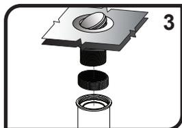
3) Securely waste line. This procedure will vary depending on the type of waste line being used. Use the included 1 1/4" adapter if needed, if not, it may be discarded. Use Teflon tape (not included) on the threads to prevent leaks.
