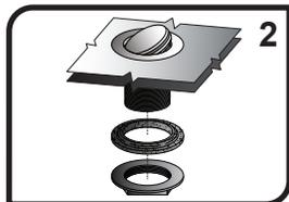
2) From under the sink, verify the overflow intake holes on the flip body assembly properly align with the overflow gap in the sink. Overflow intake holes should not extend below the gap, or water may leak out from the intake holes. Slide the thick rubber gasket up onto the threaded flip body assembly. Screw the lock nut onto the flip body assembly and tighten.
