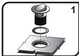
1) Set the flip body assembly with the thin gasket in the drain hole in the sink. NOTE: The thin gasket is supplied for your convenience, however, we recommend using plumber's putty (not included) instead of the gasket. Do not use both the gasket and plumber's putty.
