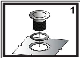
1) Set the flip body assembly with the thin gasket in the drain hole in the sink. NOTE: The thin gasket is supplied for your convenience, however, we recommend using plumber's putty (not included) instead of the gasket. Do not use both the gasket and plumber's putty.
