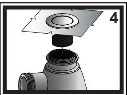
4) Screw the trap body with the adapter installed onto the threaded flip body assembly. Make sure the side port of the trap body is pointed in the desired direction for connecting the waste line, rotate complete assembly if needed. Tighten lock nut.
