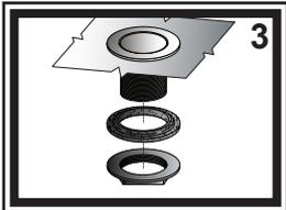
3) From under the sink, slide the thick rubber gasket up onto the threaded flip body assembly. Screw the lock nut onto the flip body assembly, but do not tighten completely.
