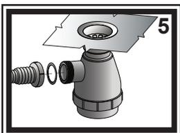
5) Securely screw the hose barb onto the side port of the trap body, ensuring the rubber gasket is properly seating inside the head of the hose barb. Slide 3/4" or 1" ID hose all the way onto the hose barb. Secure hose with a stainless steel hose clamp (not included).
