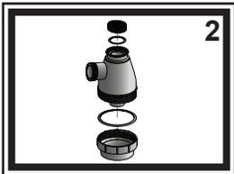
2) Ensure the trap cup and the adapter are tightly screwed onto the trap body with the rubber gaskets inside the connections.
