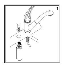
(1) Insert the bottle, with the brass shaft, lock nut, and washer, up from below. From the top, set the escutcheon onto the brass shaft. Tighten the housing down onto the shaft. Tighten the lock nut under the sink.
