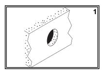
(1) Hold elbow on the wall where desired. Make sure to leave enough room for your hose to hang freely and extend into the shower. Drill 1" hole in the bulkhead in the desired location.
