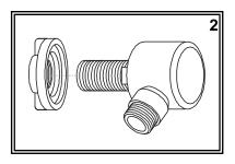
(2) Make sure male nipple is tight into the elbow with Teflon (Plumber's) tape. Slip nipple through the hole in the bulkhead. Make sure gasket properly lines up with the back of the elbow. From the back side of the bulkhead, thread the lock nut onto the brass nipple and tighten.
