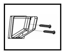
1) Mount bulkhead bracket with the two stainless steel screws provided. The top of the bracket is the side with the larger diameter opening.
