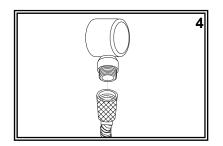
(4) Attach your 1/2" hose to the connector. Turn the water supply on. While water is running, check all connections for leaks. Connections may need re-tightening.
