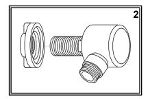
(2) Make sure male nipple is tight into the elbow with Teflon (Plumber's) tape. Slip nipple through the hole in the bulkhead. Make sure gasket properly lines up with the back of the elbow. From the back side of the bulkhead, thread the lock nut onto the brass nipple and tighten.
