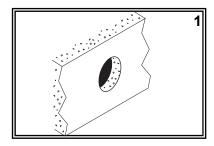
(1) Hold elbow on the wall where desired. Make sure to leave enough room for your hose to hang freely and extend into the shower. Drill 1" hole in the bulkhead in the desired location.
