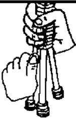
(6) Very gently bend the copper water inlet tubes slightly out, to allow for larger hose clearance. **CAUTION: USE CARE WHEN BENDING THE TUBES.** Grip at point of bend with one hand and adjust with the other. **NOTE: Damaged tubes void your warranty.**
