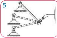
(5) Adjust the height and angle of your new extension arm as desired. Simply loosen the wingnut(s), adjust and retighten.
