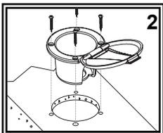
**Wall Mount**—Place into the hole with the hinge pointing DOWN. This will allow the lid to fall out of the way of the item installed inside the cup when in use. Secure recessed cup and lid using the provided four (4) screws.
