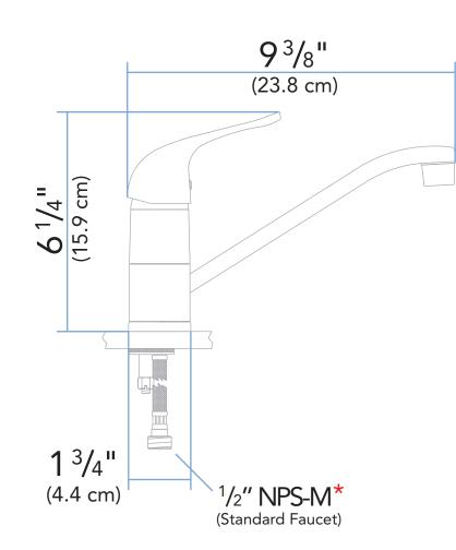
$\label{eq:linear} \begin{array}{l} \text{ALL DIMENSIONS $\pm $^{1}$ 16'' \\ \text{SOME COMPONENTS MAY NOT BE DRAWN TO SCALE} \\ \text{Ambassador Marine Inc. reserves the right to make product specification changes and to change or discontinue models without notice or obligation \\ \end{array}$
