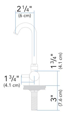
$\label{eq:linear} \begin{array}{c} \text{ALL DIMENSIONS $\pm 1^{1}$} \text{i}^{\prime\prime} \text{i}^{\prime\prime} \\ \text{SOME COMPONENTS MAY NOT BE DRAWN TO SCALE} \\ \text{Ambassador Marine Inc. reserves the right to make product specification changes and to change or discontinue models without notice or obligation} \end{array}$
