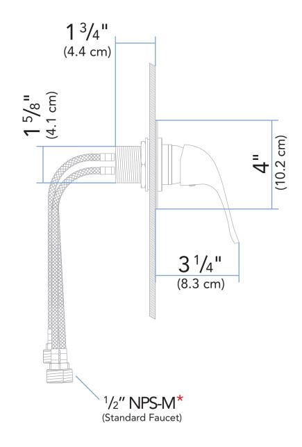
$\label{eq:linear} \begin{array}{c} \text{ALL DIMENSIONS \pm 1/16''}\\ \text{SOME COMPONENTS MAY NOT BE DRAWN TO SCALE}\\ \text{Ambassador Marine Inc. reserves the right to make product specification}\\ \text{changes and to change or discontinue models without notice or obligation} \end{array}$
