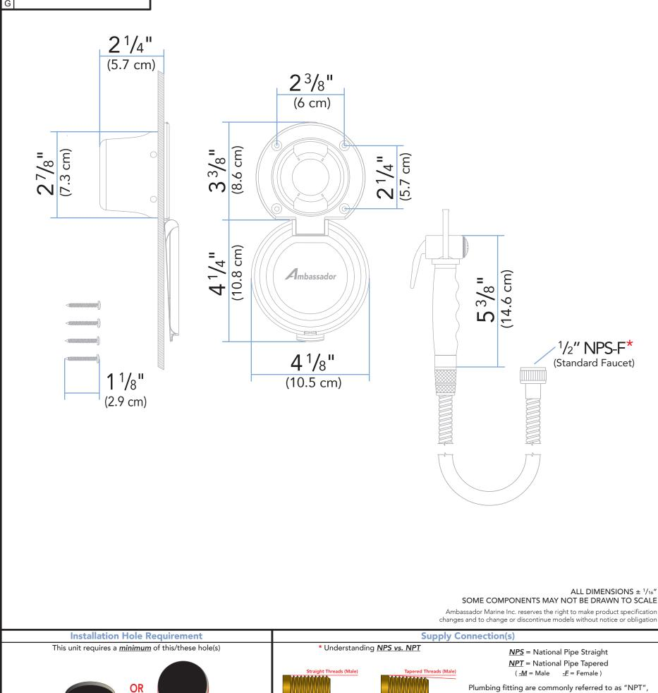
Plumbing fitting are commonly referred to as "NPT", however, in reality, nearly all faucets are actually "NPS". NPS is the North American "<u>STANDARD</u>" for faucets, regardless of brand, style, application, etc. Outside North America, BSP is the most commonly used standard.
